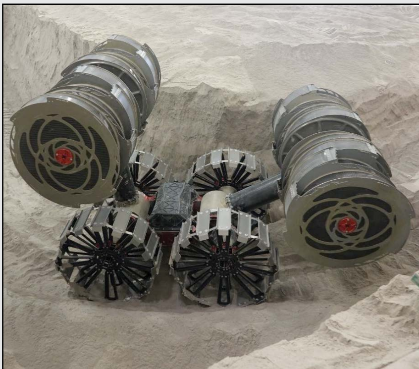
Excavator designed for lunar use undergoing testing at the NASA Kennedy Space Center. Photograph from Keszthelyi and others (2023), used with permission.
