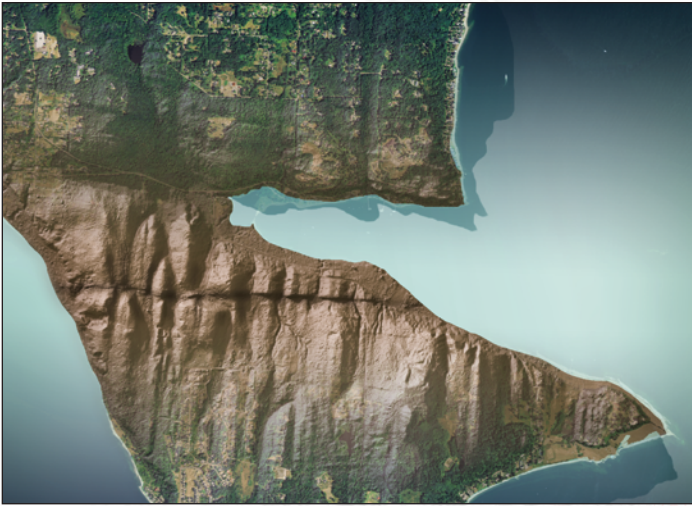
Blended and modified aerial hillshade image of Bainbridge Island, Washington, showing sharp breaks in topography from earthquake rupture on the Toe Jam Hill Fault, which is part of the Seattle Fault Zone. Images from Washington Geological Survey (Washington State Department of Natural Resources), used with permission.
