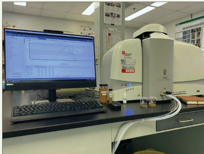
Figure 2. Photograph of laser diffraction equipment used for particle-size analysis. Photograph by Grant Colip, U.S. Geological Survey.
