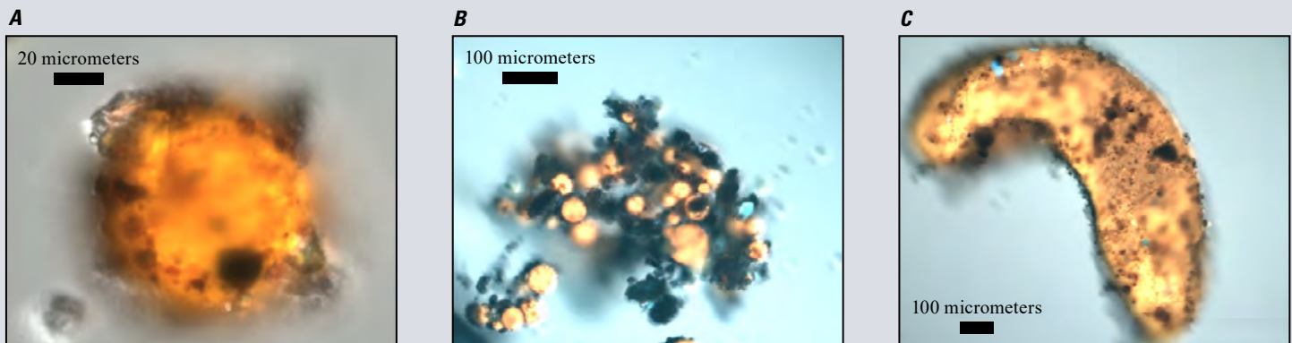
Figure 4. Images showing different types and sizes of oil-particle aggregates (OPA) from Cold Lake Blend diluted bitumen and Kalamazoo River sediment from laboratory experiments with a range of mixing energy. Oil is golden color; sediment is black. A , Single droplet-type OPA; B , Aggregates of droplet-type OPA; C , Irregular-shaped solid-type OPA (images modified from Waterman and Garcia [2015]).
