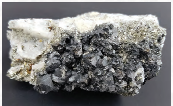
Photograph of sphalerite with pyrite, sampled from the C-East pushback, Continental Pit, Butte Mining District, southwestern Montana. Photograph from Kyle Eastman, Montana Technological University.
