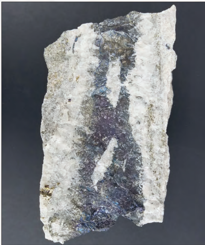
Photograph of chalcocite-bornite-pyrite Main Stage vein, sampled from the C-East pushback, Continental Pit, Butte Mining District, southwestern Montana. Photograph from Kyle Eastman, Montana Technological University.
