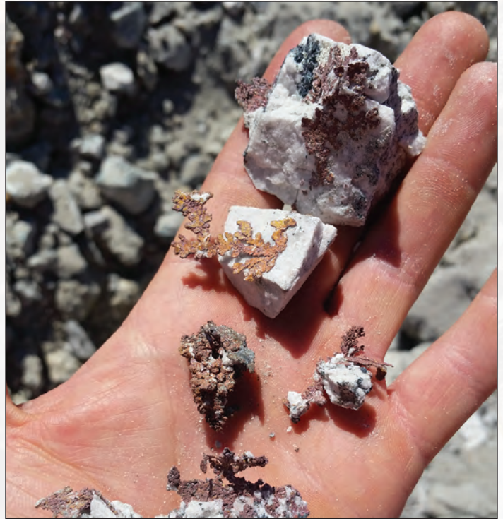
Photograph of native copper, sampled from the D-North pushback, Continental Pit, Butte Mining District, southwestern Montana. Photograph from Kyle Eastman, Montana Technological University.
