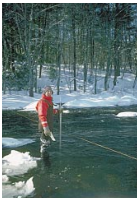
Figure 4. A technician measures the velocity and volume of streamflow in the Lamprey River.
