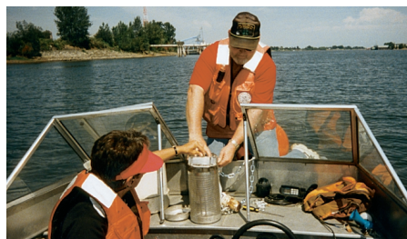
Figure 2. USGS hydrologists prepare to deploy a semipermeable-membrane sampling device in the Columbia River.
