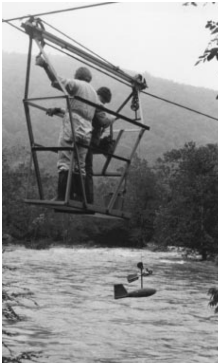
Figure 2. Measurement of surface-water flow from a cable suspended above a stream.
