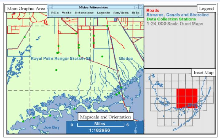
Figure 1. Map graphic of a portion of South Florida showing the main graphics area, map scale and orientation box, legend information area and overview inset map generated by a GIS interface developed by the U.S. Geological Survey (USGS). This illustrates the framework of what a user sees on the computer screen when running the GIS graphical user interface called DBView.
