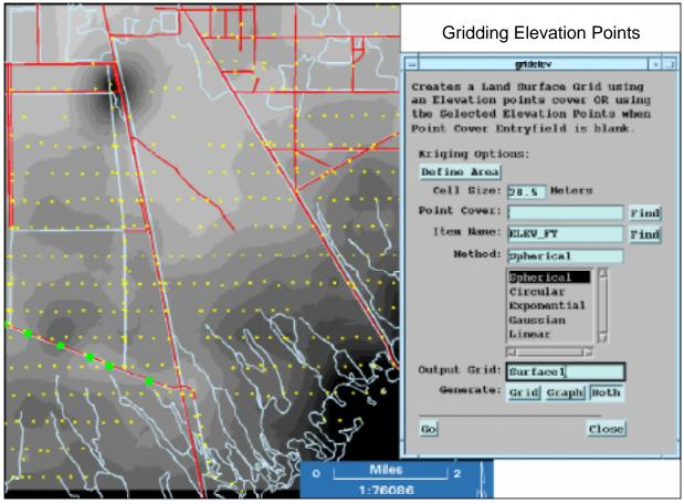
Figure 3. Contour map generated and displayed by DBView showing roads (red lines), elevation data points (yellow dots), and streams, canals, and shoreline (blue lines). Lighter colored areas indicate higher land-surface elevations whereas darker colored areas indicate lower elevations.
