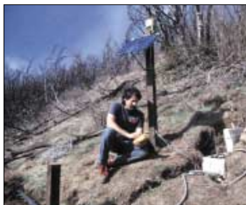
Above: Testing a solar-powered radio telemetry system for remote transmission of real-time landslide data (Photo: Mark Reid, USGS)
