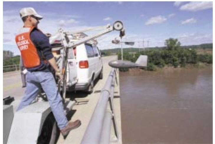
Checking the health of the Nation's rivers. Measuring flow from a bridge near a USGS streamgage.
