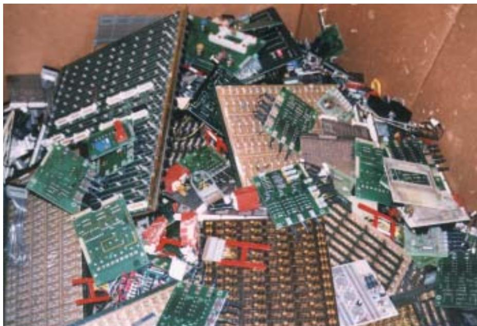
**Figure 1.** Circuit boards are sought after by recyclers for their metals content, especially gold and silver. Photograph courtesy of Melissa Goodrich, Recycling Today.
