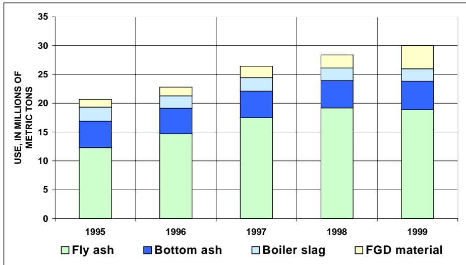
Figure 3. Amounts of coal combustion products used in the United States, 1995-99. Data from the American Coal Ash Association.
