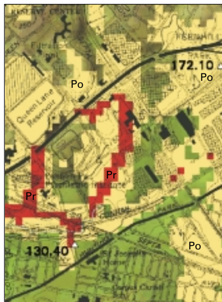
Figure 5. Examples from the topographic change map included in USGS Open-File Report 00-224. Areas shaded in yellow and labeled Po have been characterized as possible fill. Areas shaded in red and labeled Pr have been characterized as probable fill. A, Map segment showing historical stream valleys of Wissinoming Creek and Little Tacony Creek. B, Map segment showing historical stream valley of Wingohocking Creek. C, Map segment showing small creek beds and topographically low areas and possible fill along rail lines and interstate highways.
