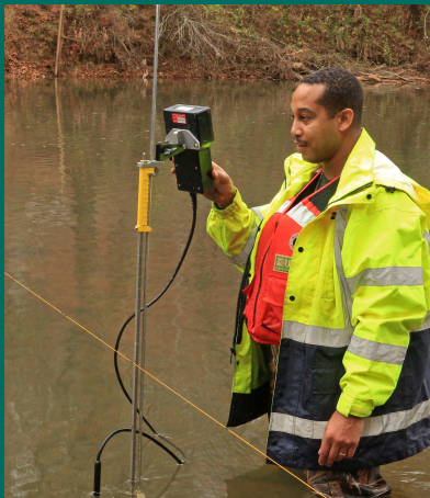
USGS hydrologic technician making a wading streamflow measurement. Photograph by Alan Cressler, U.S. Geological Survey.
