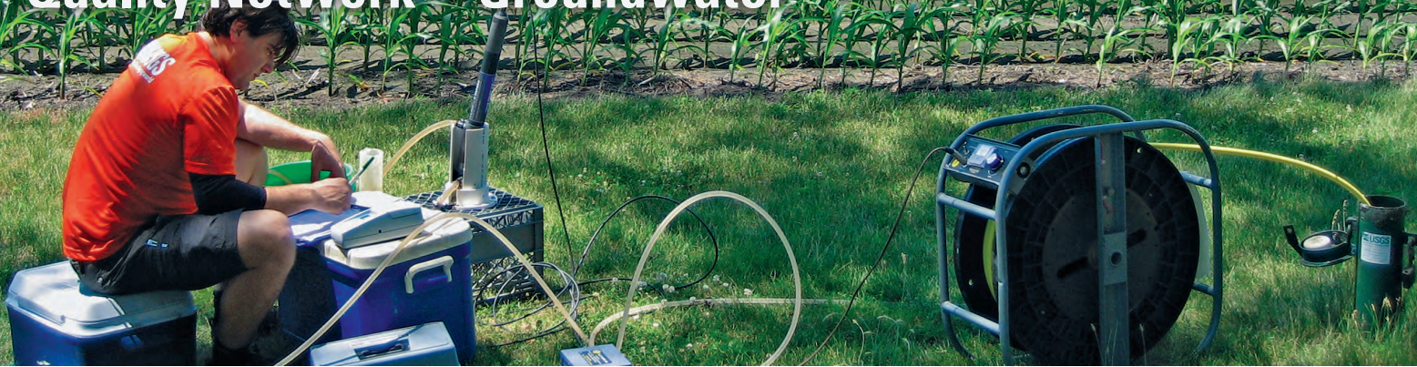
USGS scientist sampling a monitoring well in an agricultural setting. Photograph by William Morrow, USGS.
