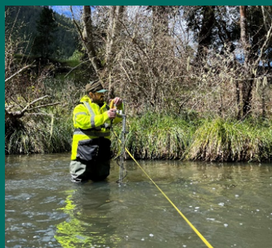
USGS hydrologic technician measuring streamflow at USGS streamgage Cow Creek near Azalea, OR (14309000). Photo by Georgia Michael, USGS.
