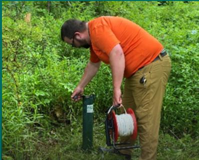
USGS hydrologic technician making a groundwater measurement at a USGS monitoring well in Southbury, Connecticut (USGS station 412935073122701). Photograph by USGS.
