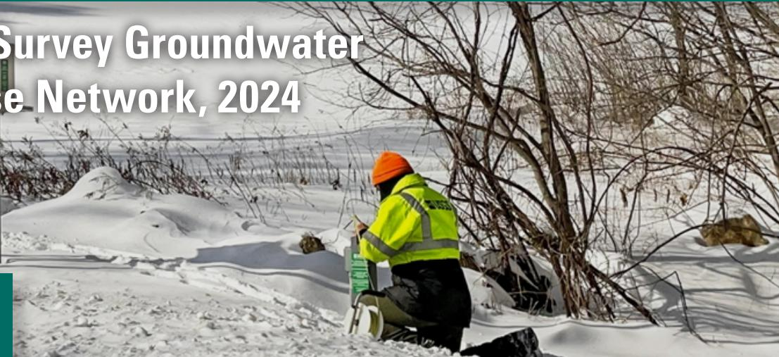
USGS hydrologic technician making a groundwater measurement in Montgomery, Massachusetts (USGS station 421240072490201). Photograph by Samuel Banas, USGS.
