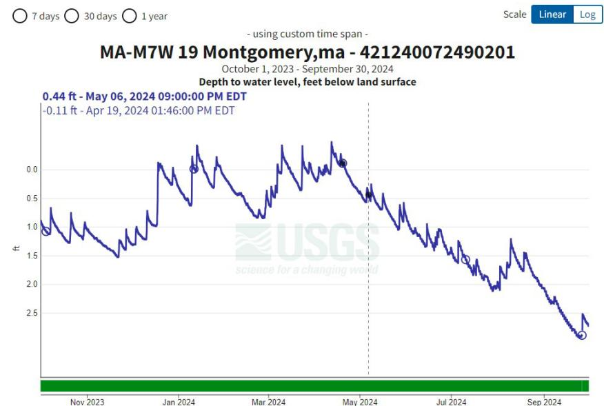
Groundwater hydrograph from a Climate Response Network well in Montgomery, Massachusetts (USGS station 421240072490201), October 1, 2023 to September 30, 2024. Accessed January 10, 2025, at <https://waterdata.usgs.gov/monitoring-location/421240072490201/>.
