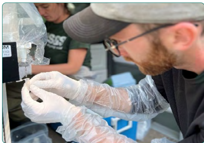
U.S. Geological Survey (USGS) hydrologic technician processing per- and polyfluoroalkyl substances samples from the Delaware River at Trenton, NJ (USGS station 01463500). Photograph by Pamela Reilly, USGS.
