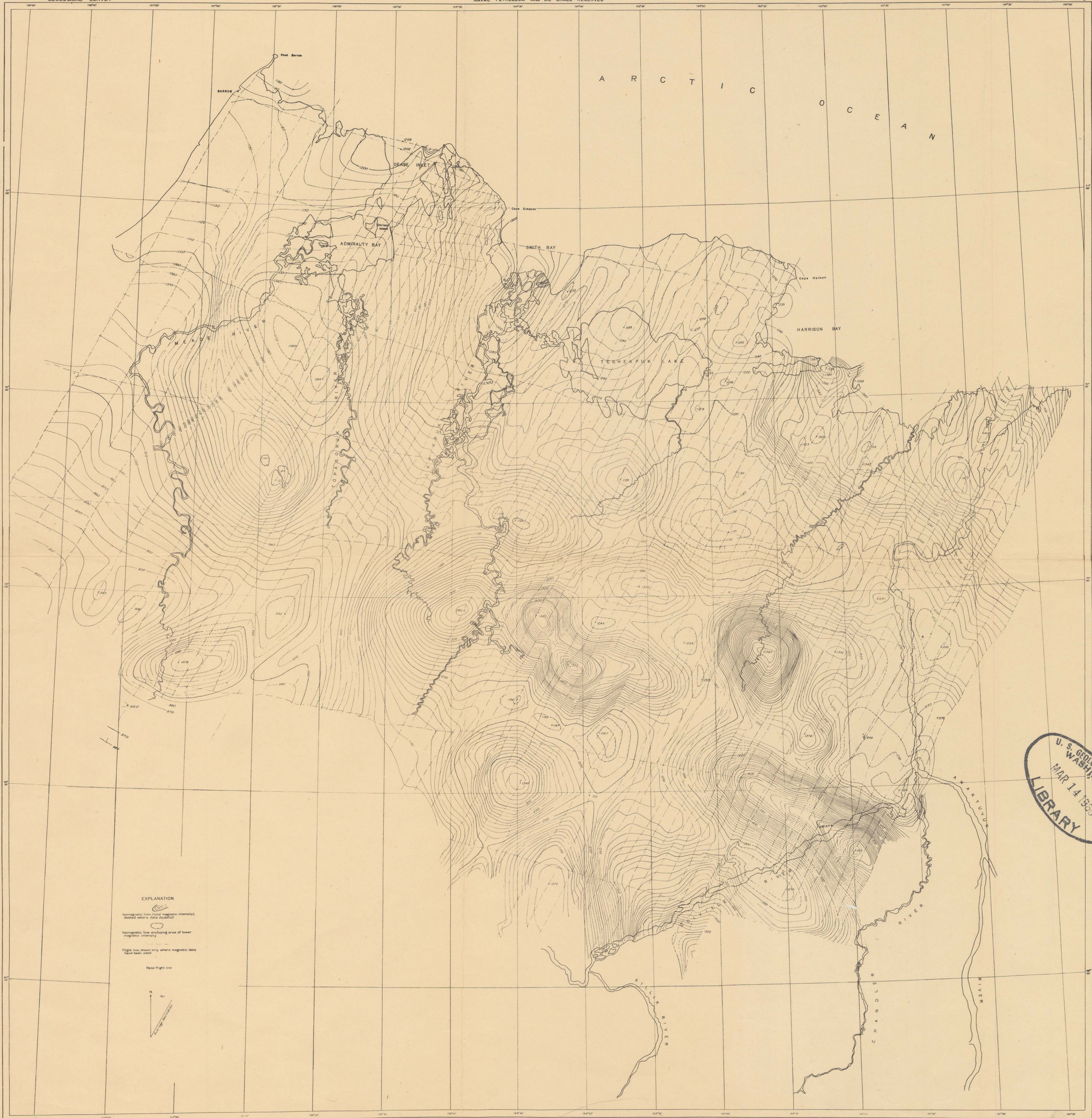
PLATE 3 PRELIMINARY MAP SHOWING TOTAL MAGNETIC INTENSITY IN PART OF NAVAL PETROLEUM RESERVE NO. 4, ALASKA
