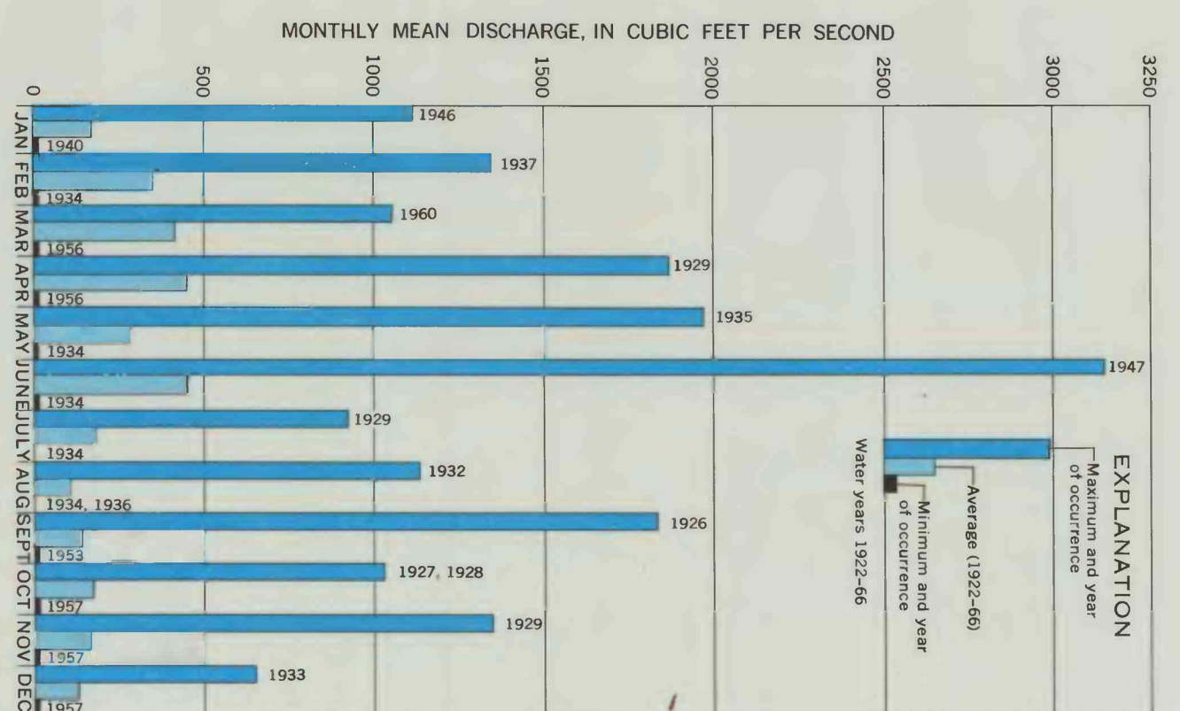
THE POSSIBILITY OF LOW STREAMFLOW CONDITIONS OCCURRING IN MONTHLY MEAN DISCHARGE OF NORTH MISSOURI IS INDICATED BY THE UNSTABILITY OF STREAMFLOW AS A PERENNIAL SOURCE OF SUPPLY. DISCHARGE WAS LOW IN JULY AND AUGUST 1933 AND IN AUGUST 1936.
