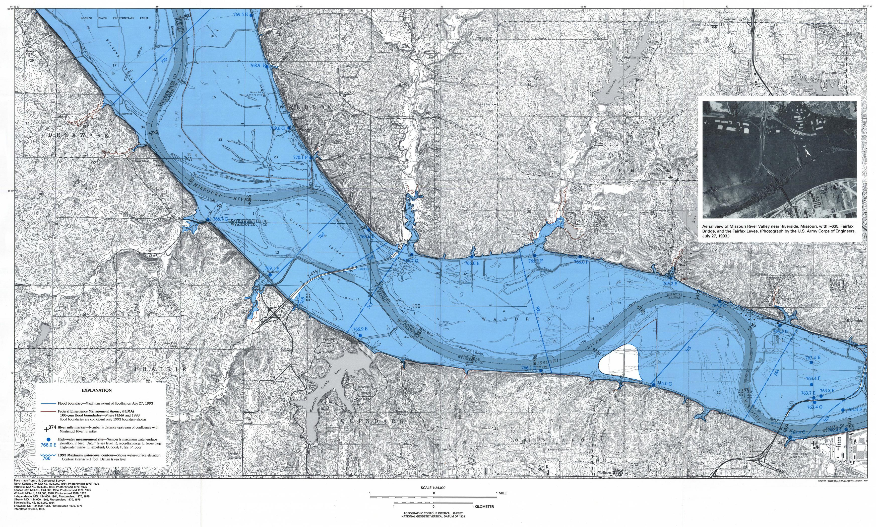
Figure 1A. Flood boundaries, water-elevation measurements, and water-level contours for 1993 and Federal Emergency Management Agency 100-year flood boundaries for the Kansas City metropolitan area from about Missouri River miles 390 to 373.
