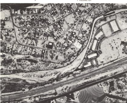
Figure 3.—Santa Cruz River upstream from Grant Road. The constriction at point A on the photograph may cause water to flow over the bank at point B; the water would flow through the industrial park, and buildings would be subject to erosion during major floods. The arrow indicates the direction of flow. Scale: 1 in. = about 800 ft.
