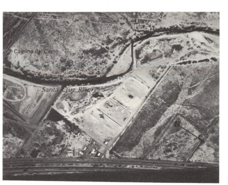
Figure 2.—Gravel pits along the Santa Cruz River in sec. 17, T. 13 S., R. 13 E., about 2,000 ft north of Camino del Cerro. Note how the channel is diverted to the west by the dike around the northernmost pit. This type of channel constriction is common along the river. The arrow indicates the direction of flow. Scale: 1 in. = about 650 ft. Photograph furnished by Cooper Aerial Survey Co.
