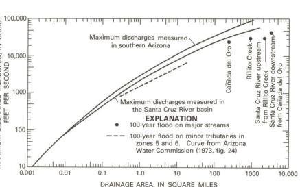
Figure 1.—Relation of maximum discharge measured to size of drainage area.
