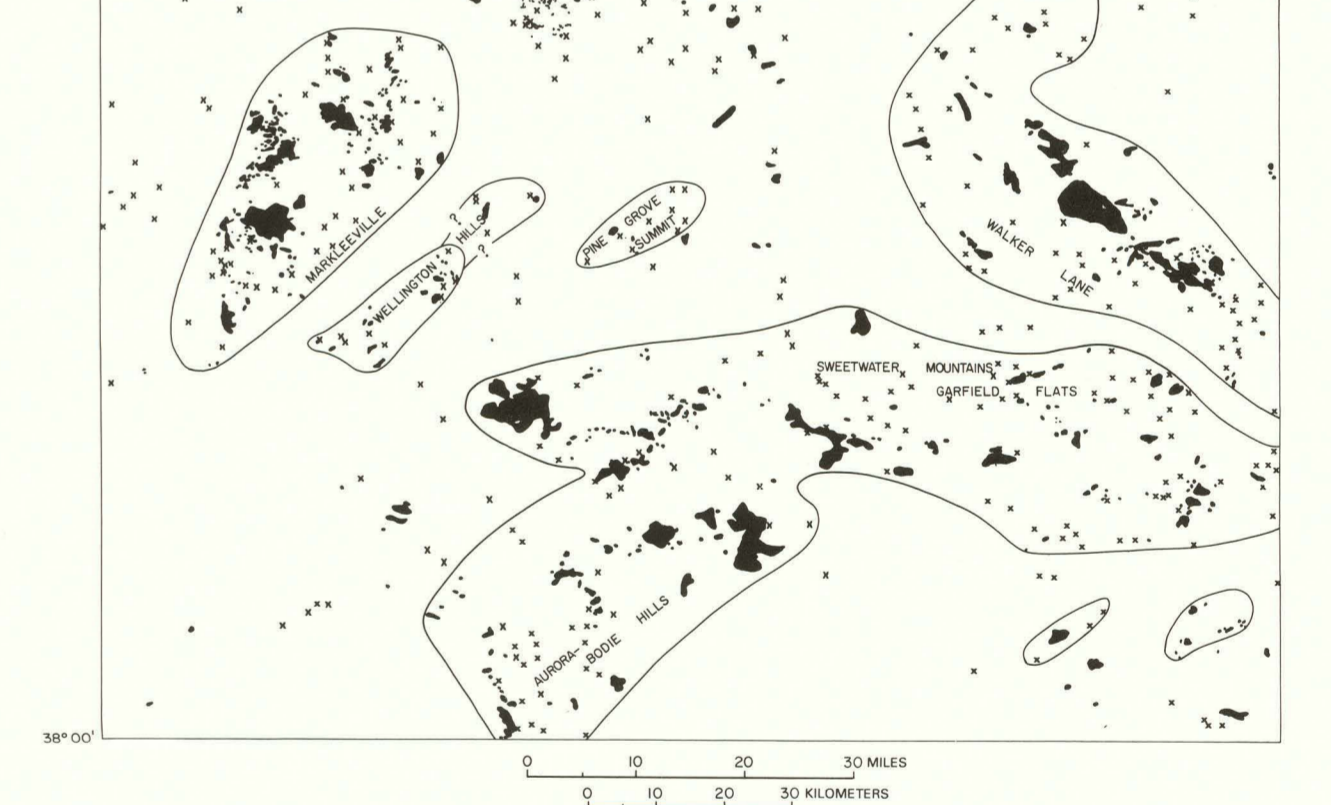
FIGURE 3.—Map showing the distribution of both hydrothermally altered rocks and mines and prospects where altered rocks were not mapped. Belts of hydrothermally altered rock are delineated by heavy lines. Locations of mines and prospects are indicated by X's.
