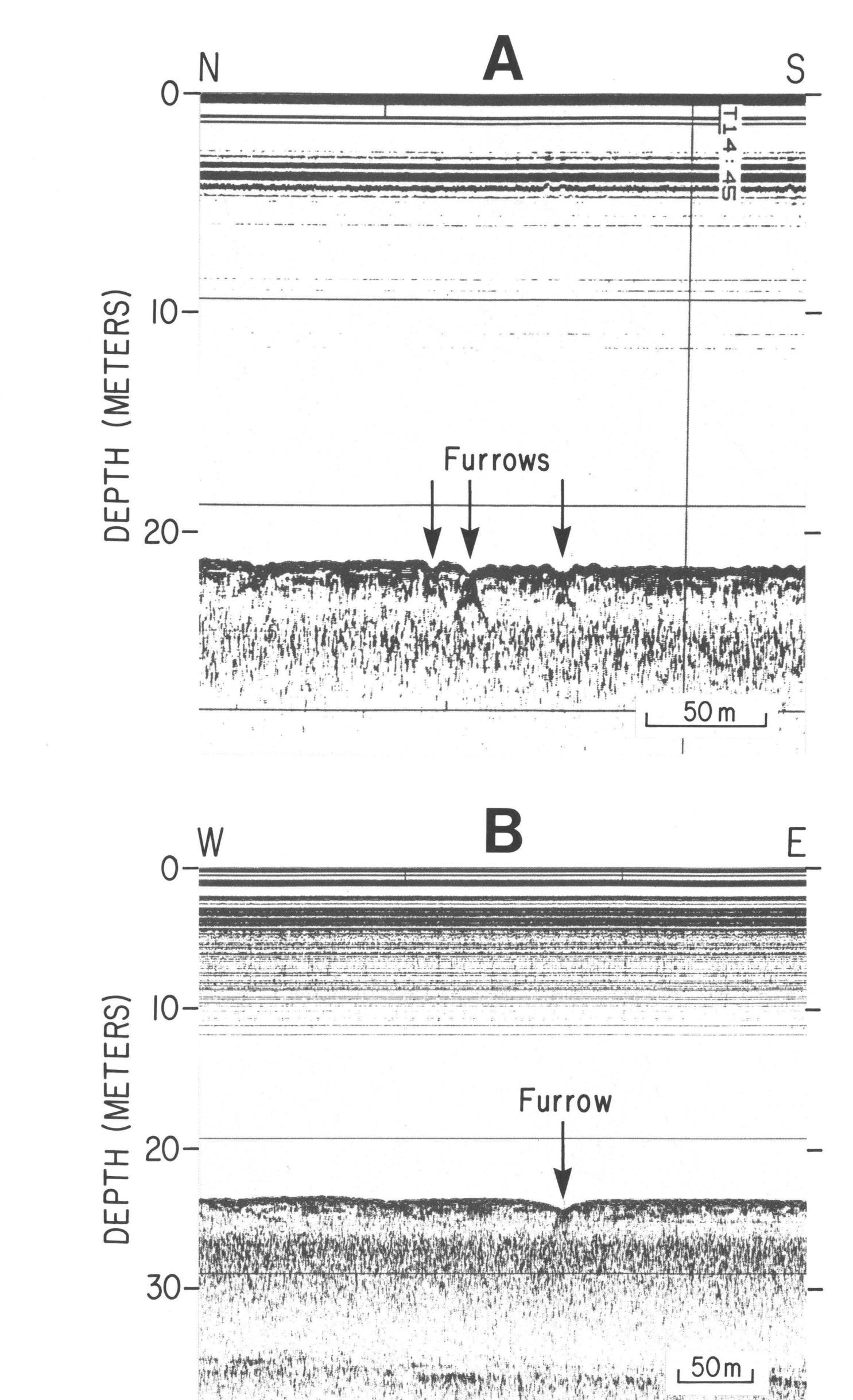
Figure 9.—Subbottom profiles in the eastern part of the New Haven Dumping Ground study area showing characteristics of sedimentary furrows. Profile locations are shown in figure 8. A, Cross section across three east-west-trending furrows, made while the vessel was turning to come on line. B, Oblique cross section of a well-developed east-northeast-trending furrow. Note slight asymmetry of the furrow walls.
