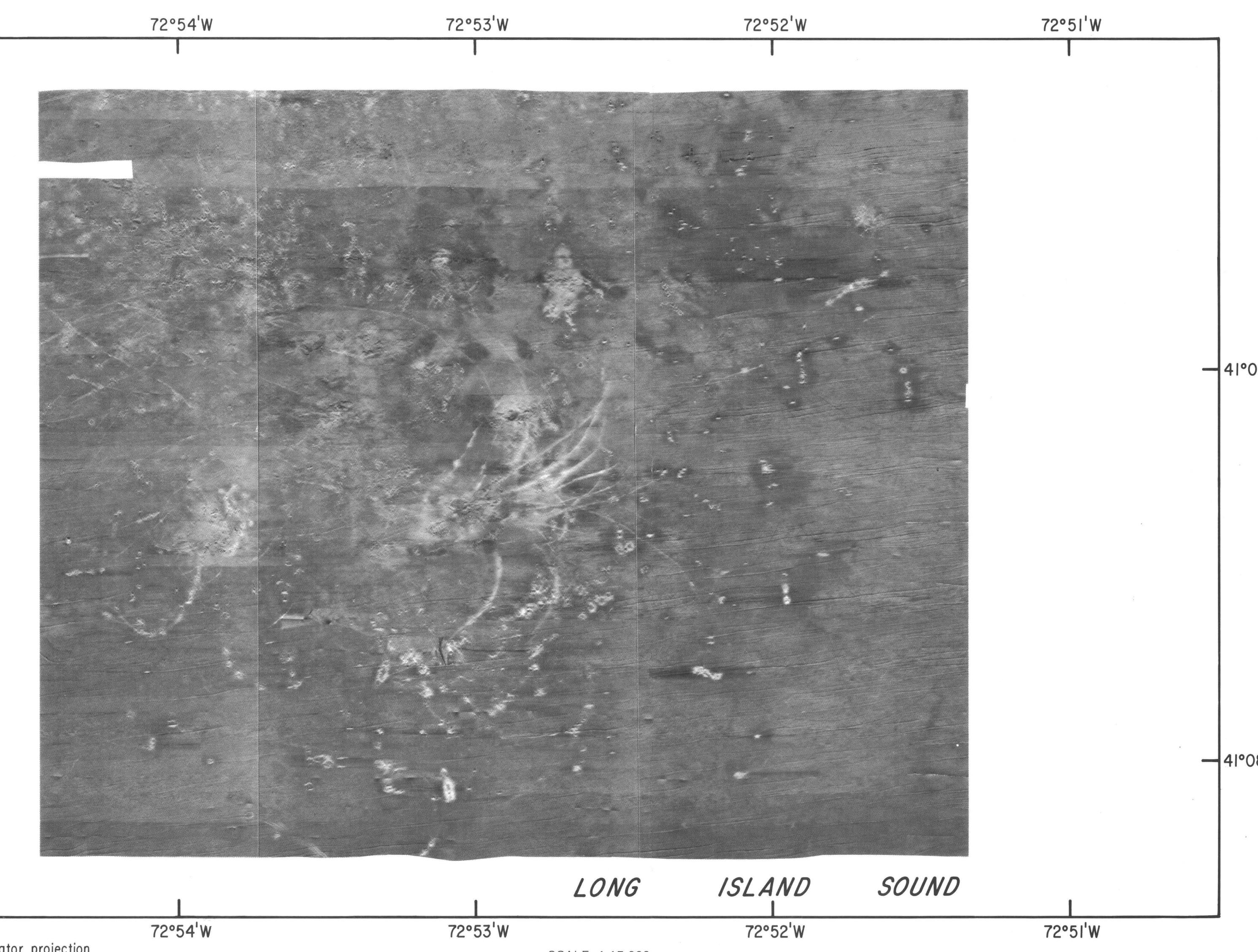
Figure 12.—Sections of sidescan sonar records from the New Haven Dumping Ground study area. Locations of sections are shown in figure 11. A, "Tuning fork" joining pattern exhibited by some sedimentary furrows. Most forks point to the east (right), suggesting net westward transport. B, Association of some furrows with piles of dredge spoils. The association of the furrows off the east and west sides of the dredge spoils is evidence for the oscillatory nature of the net westward transport.
