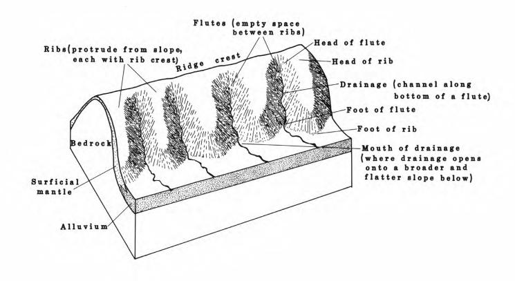
Figure 3.—Block diagram explaining the nomenclature used to describe terrain features and landslide habitats.
