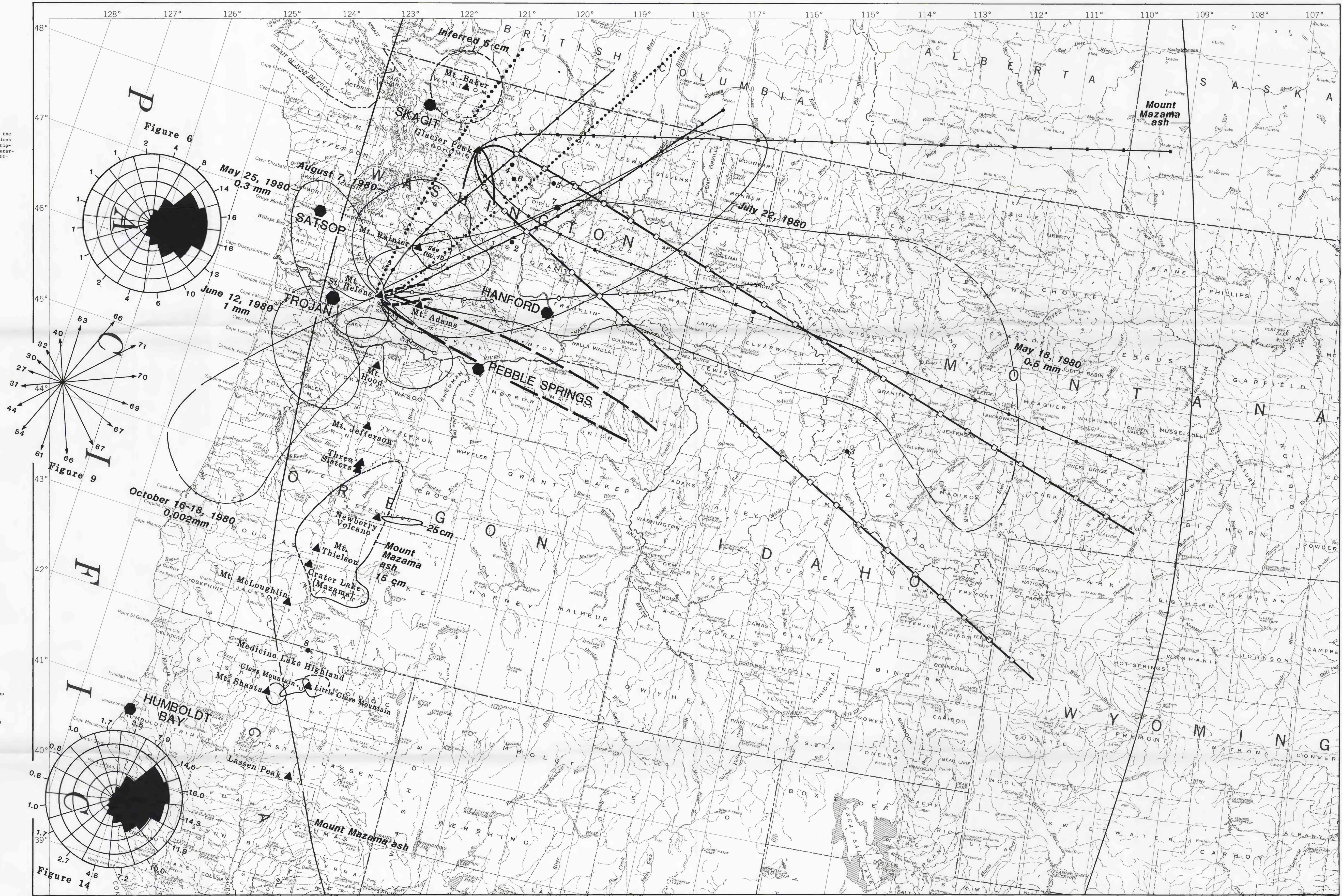
Figure 14—Percentage of time annually that winds at altitudes between 3,000 and 16,000 m (10,000–53,000 ft) blow toward sectors along main compass directions over Medford in southern Oregon (indicated by stippled pattern). Modified from Miller (1980).
