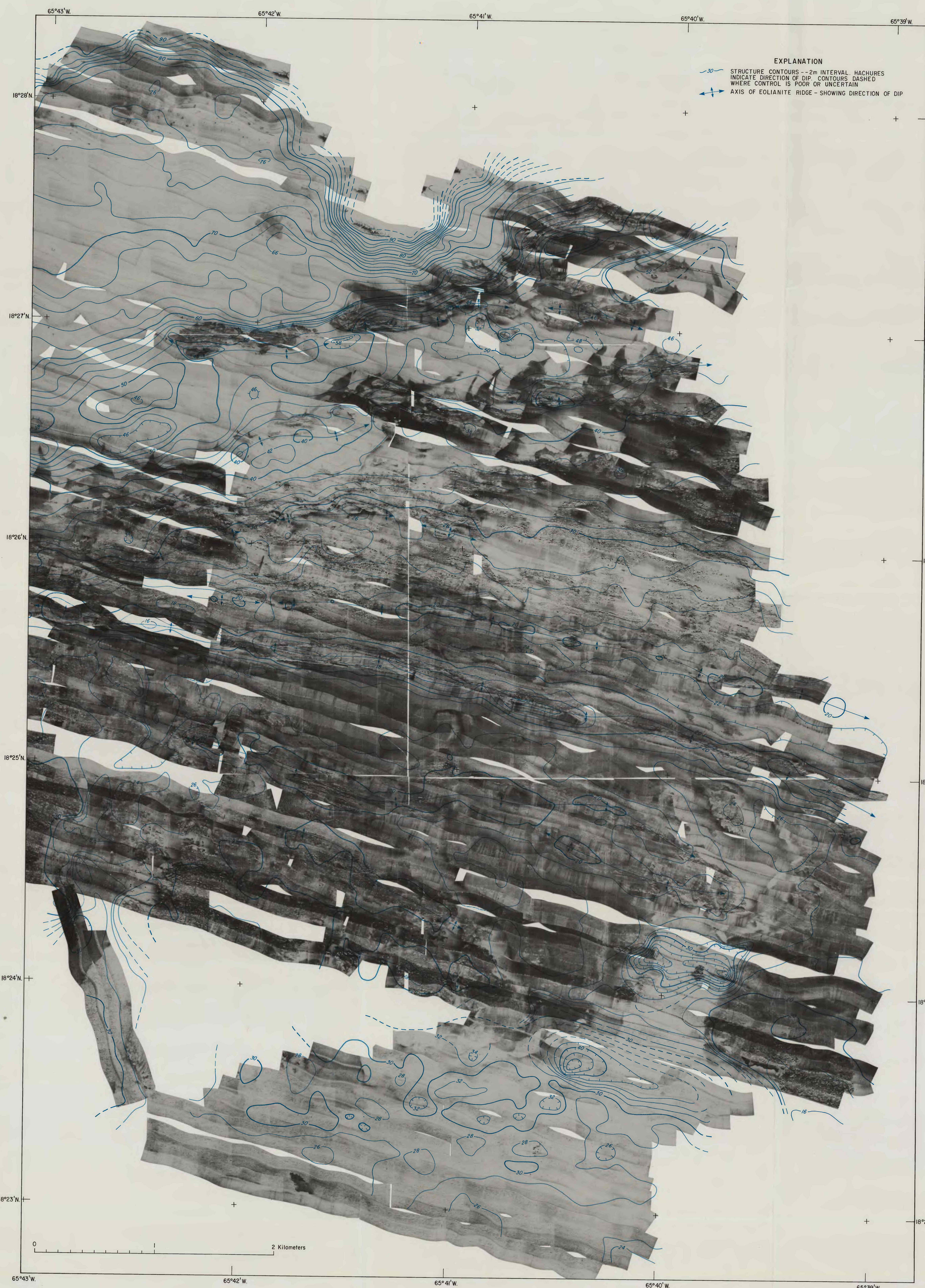
Map J. Side-scan sonar imagery collected over the eastern segment of the study area showing the structure of the Pleistocene surface and crests of eolianite ridges.
