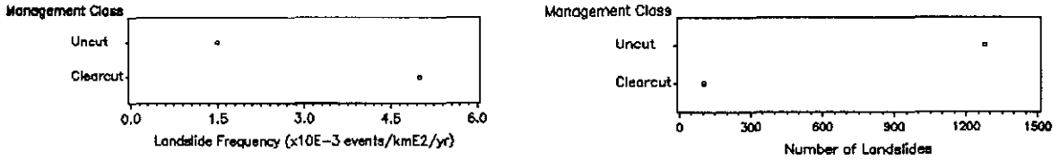
Figure 2. Comparison of landslide occurrence in cut and uncut areas in southeast Alaska based on aerial photographic analysis.
