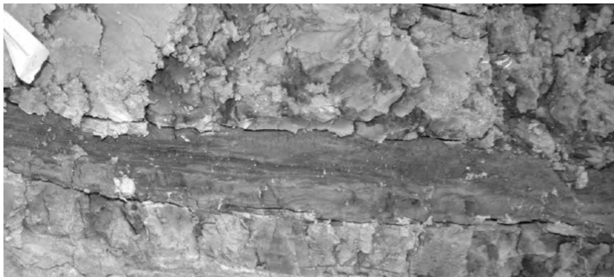
Figure 5. Example of sandy layer with charcoal layers and overlying thick dense clay deposits near Station 50.
