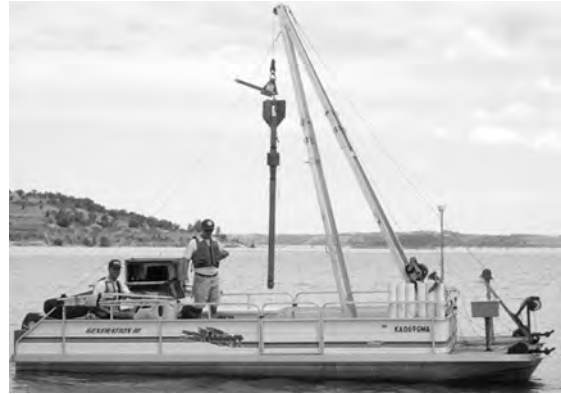
Figure 2. Bottom-sediment cores were collected with a gravity corer mounted on a pontoon boat. The corer is lowered to a designated distance above the sediment and allowed to free fall to penetrate through the entire thickness of reservoir bottom sediment.
