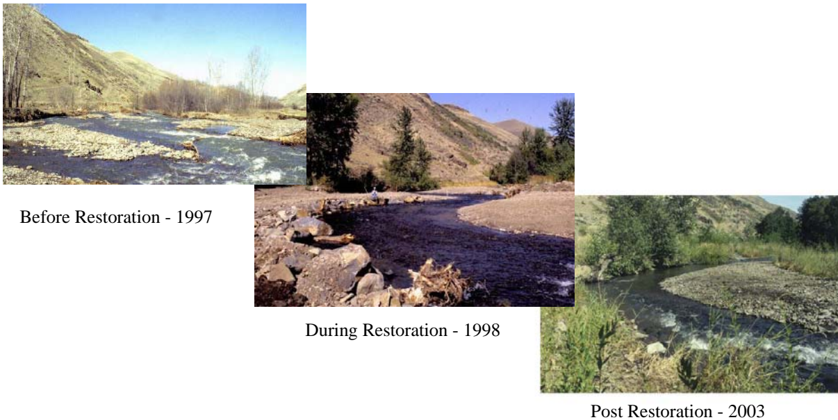
Figure 3 Geomorphic Restoration of a Braided Stream System
