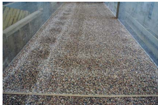
Figure 7 A series of pits in the longitudinal direction observed during the experimentation.
