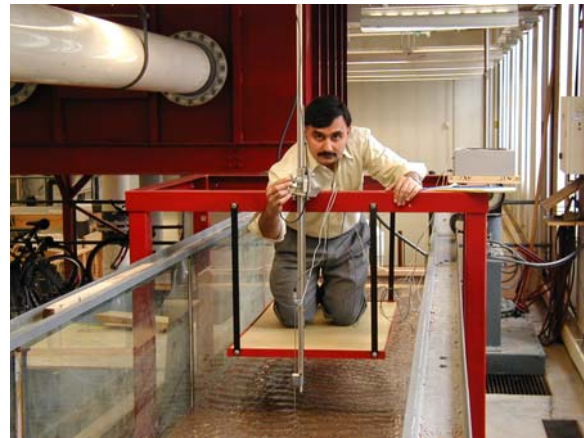
Figure 1 Measurements in progress with a flume channel in the hydraulics lab of the University of Manitoba (2003).
