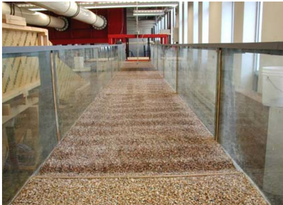
Figure 8 A wavy bed surface observed during the experimentation.
