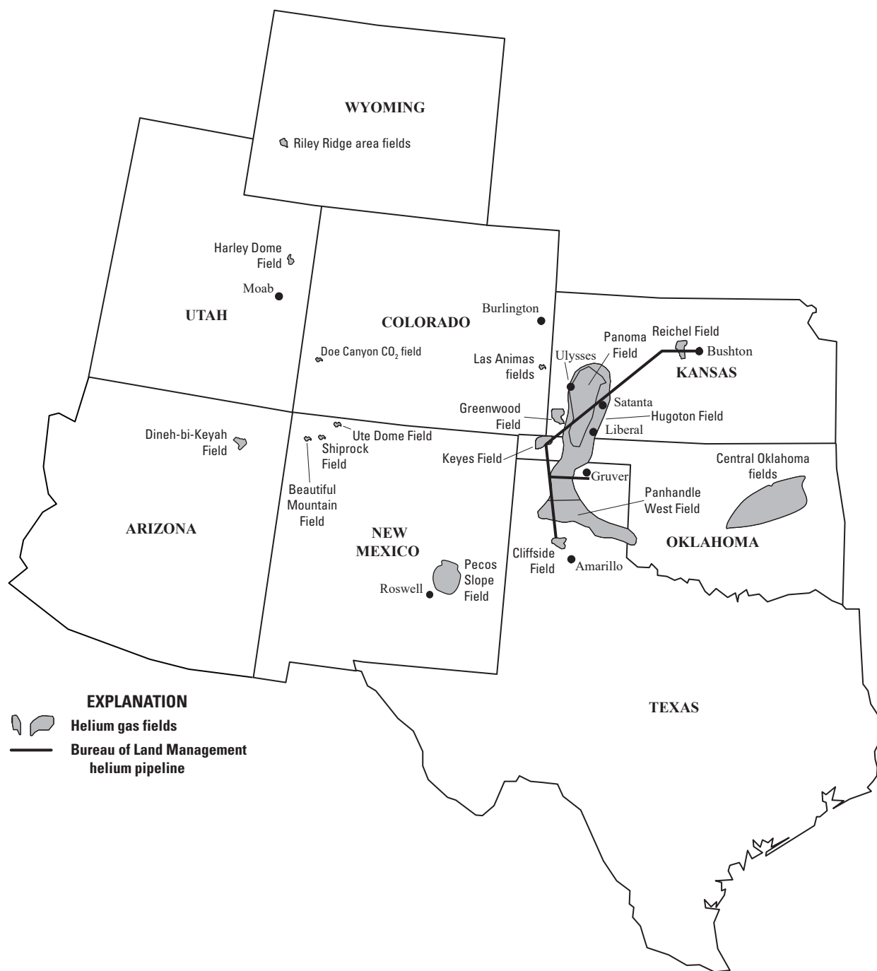
Figure 1. Major helium-bearing natural gas fields in the United States. The Panoma Field underlies the western two-thirds of the Kansas portion of the Hugoton Field.
