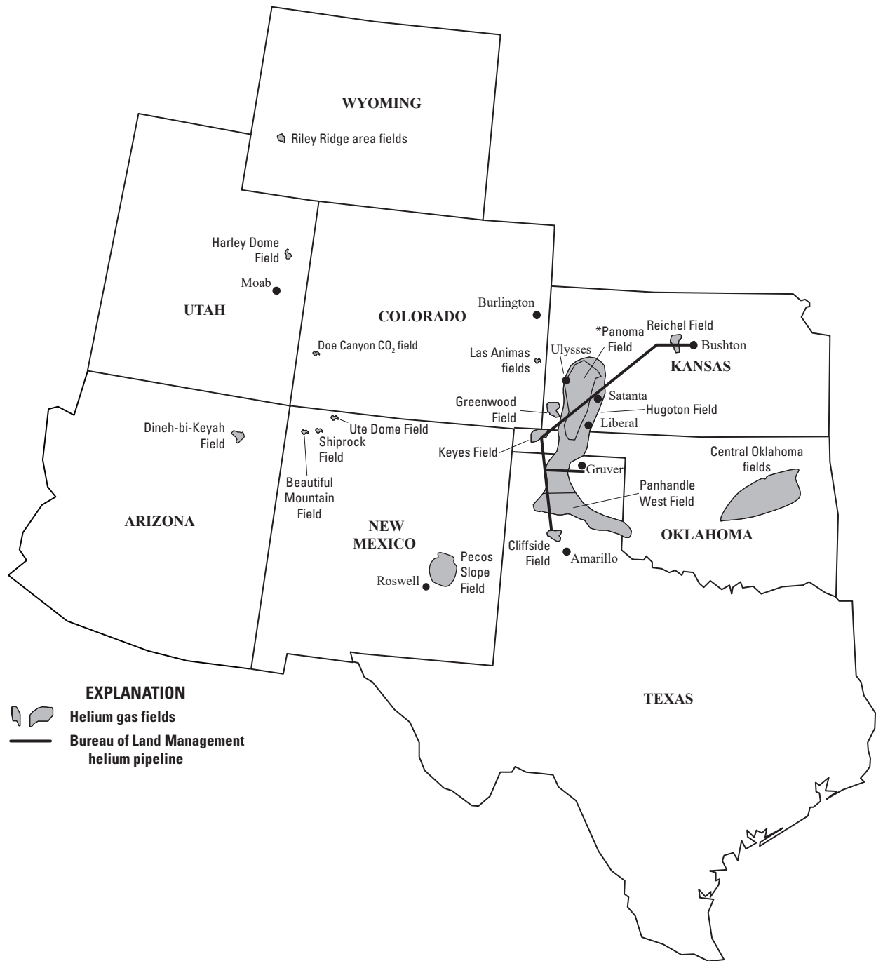
Figure 1. Major helium-bearing natural gas fields in the United States. The Panoma Field underlies the western two-thirds of the Kansas portion of the Hugoton Field. CO 2 , carbon dioxide.
