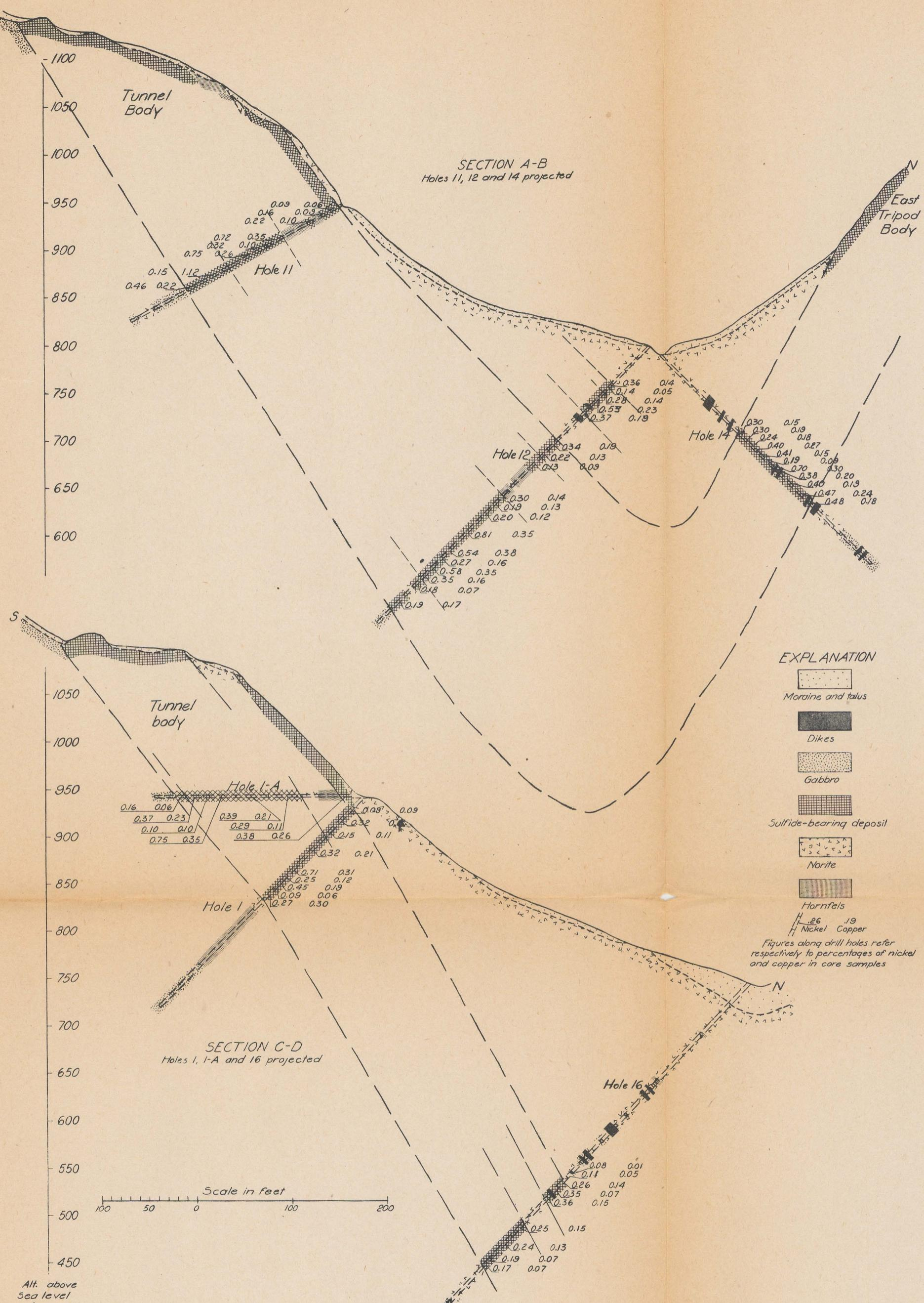
Fig. 5 Geologic sections across sulfide-bearing deposit, Yakobi Island, Alaska
