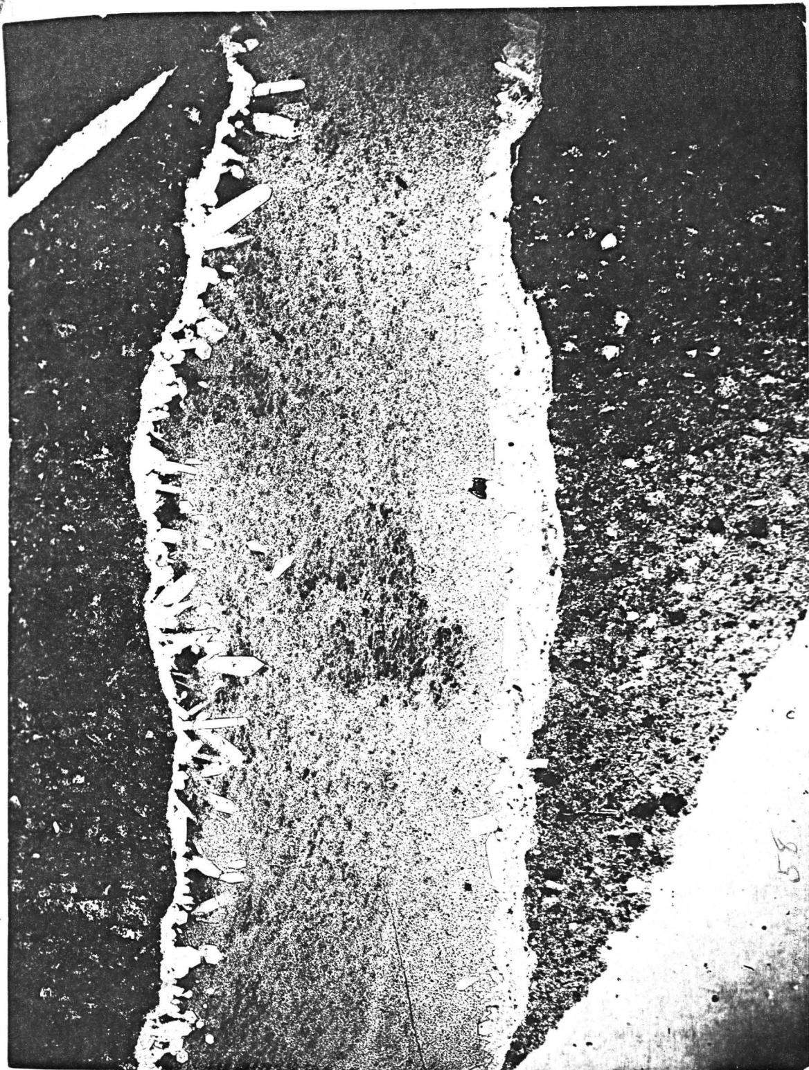
Fig. 58. Microphotograph of a section (a'-b') of the veinlet a-b in figure 57, showing it to be composed mainly of fine-grained cuboidal crystalline alunite between thin walls of mostly columnar quartz. x25 diameters. Under equally high power it is similar to figure 60.
