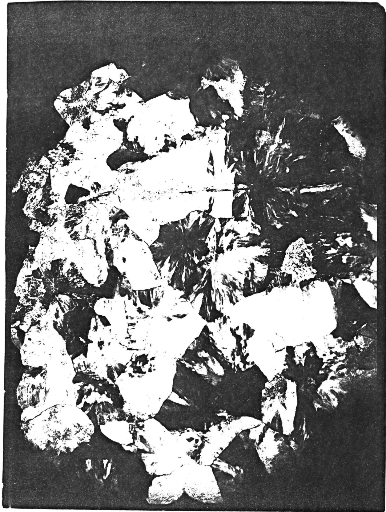
Fig. 36. Photomicrograph of ore (specimen 194) from Pyramid vein, showing flamboyant or pseudospherulitic structure in the gangue quartz. x40 diameters.
