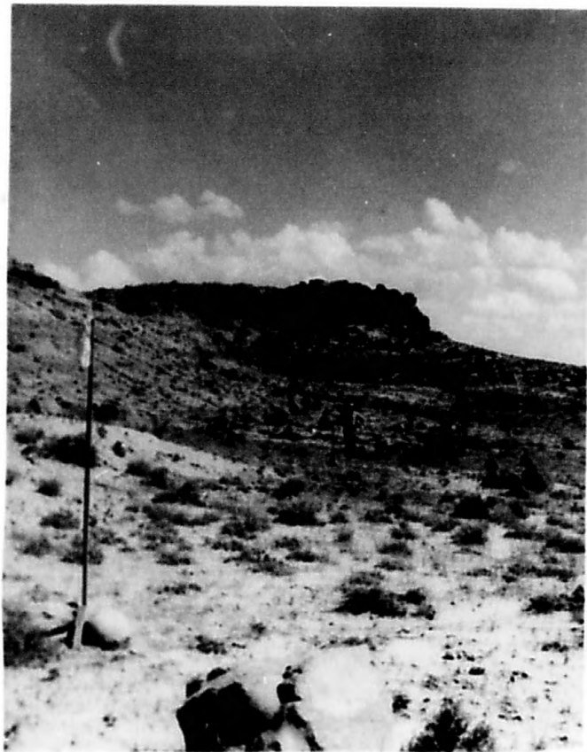
A. EROSION MEASUREMENT RANGE B-6 AT BASE OF CLIFFS. PICKET IN FOREGROUND MARKS WEST END OF RANGE. THE MAN IS STANDING NEAR A ROD MARKING THE EAST END.
