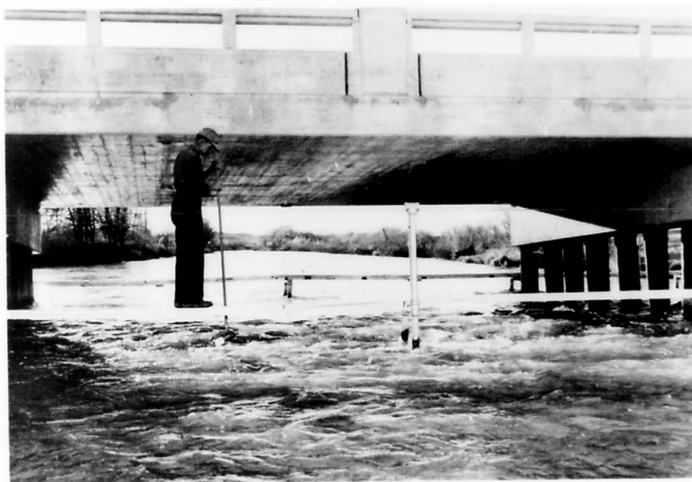
B. Center reach of section D looking upstream. Hand sampler (US DH-48) in use.
