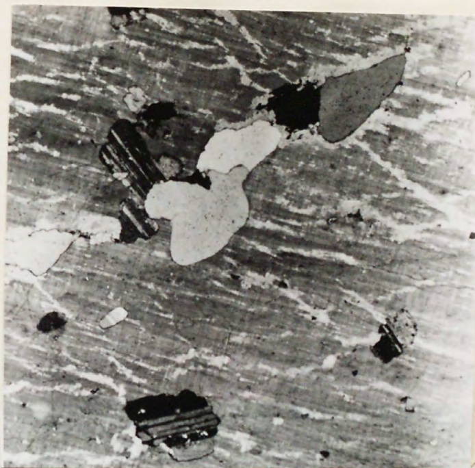
Plate 12. A, Photomicrograph of microcline perthite with albite (twinned), quartz (white to gray) and biotite (black) inclusions. Diagonal white veinlets are albite. Note narrow clear rims on albite inclusions. Some specimen as plate 11. x-nicols. 30X
