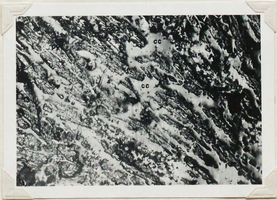
Figure 8 X-100. Polished section of chalco-cite-cc replacing pyrite-py in nodule.
