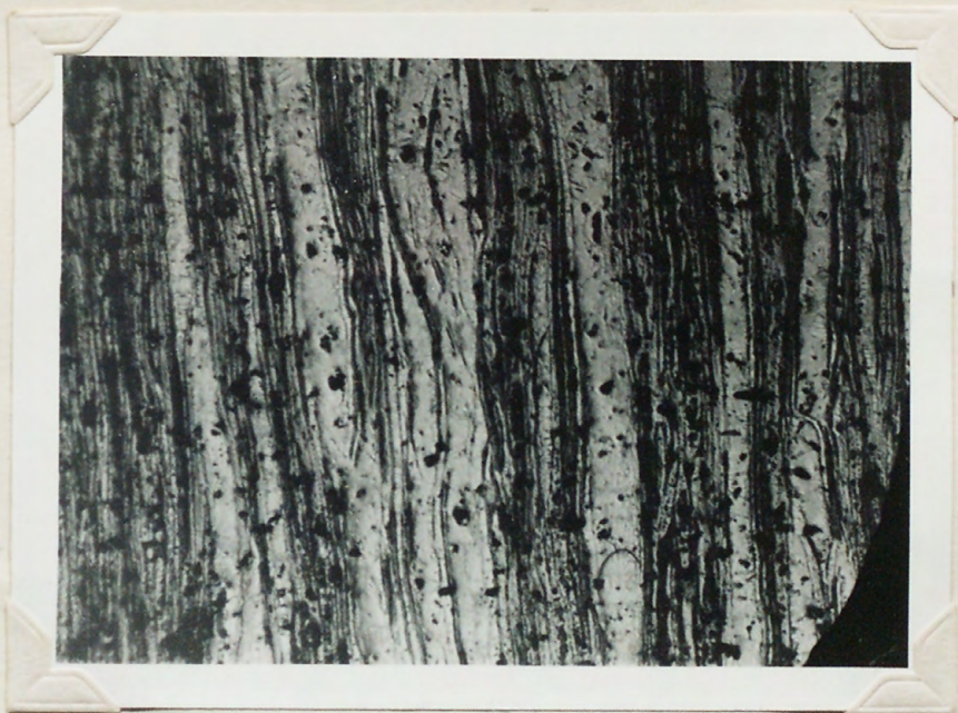
Figure 11 X-100. Longitudinal section of copper replaced wood showing cell structure.
