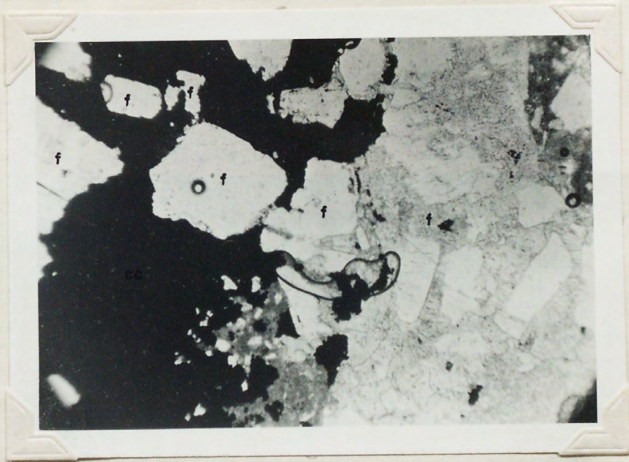
Figure 7 X-100. Thin section showing chalco-cite-cc replacing calcareous cement and feldspars-f in arkose.
