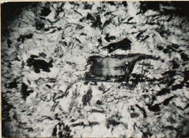
Figure 8b. Porphyritic texture in minette dike. Biotite phenocrysts in groundmass of altered orthoclase. Plane light, x 15. Location, west shore of Beaver Neck 1 mile south of Fox Hill.
