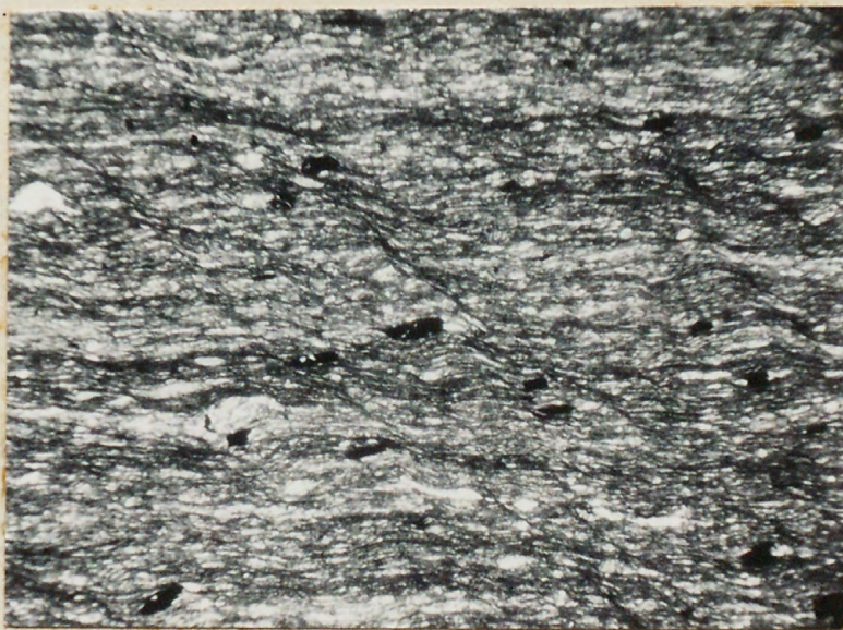
Figure 4b. Crenulated phyllite; minor folds are at angle to schistosity; rock composed chiefly of sericite, chlorite, and fine-grained quartz. Dark grains are leucoxene. Crossed nicols, x 28. Location, Fox Hill.
