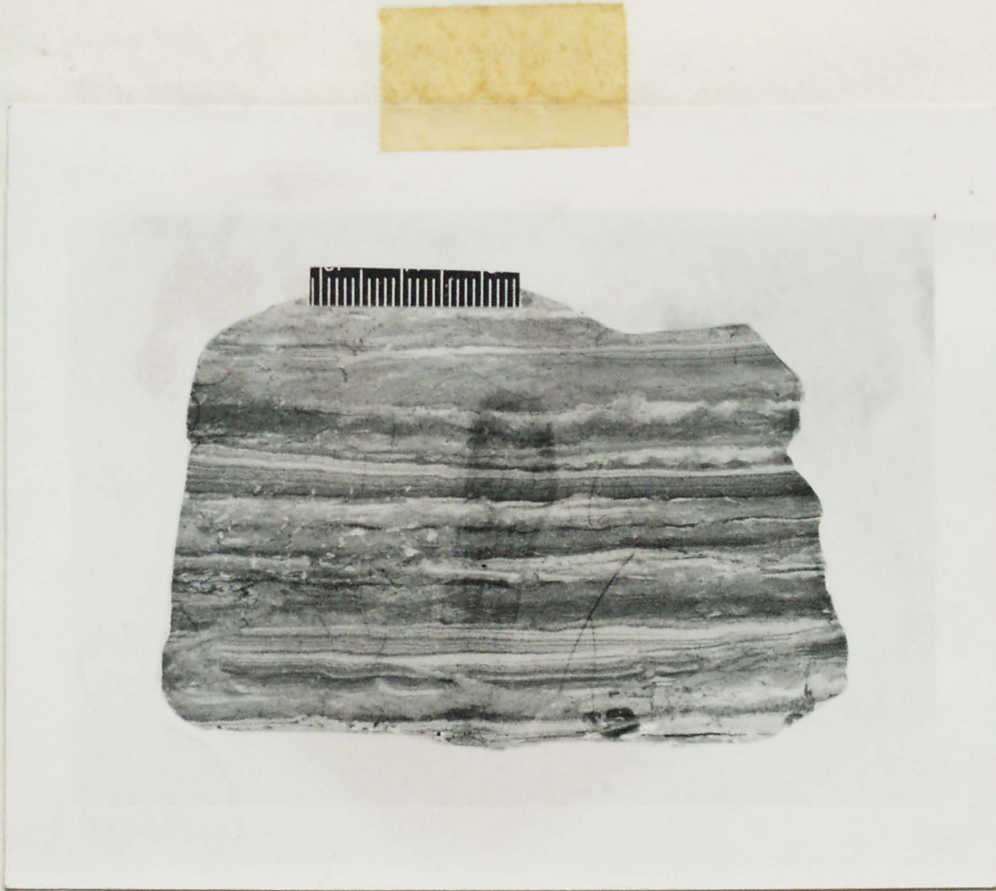
Figure 17.— Varve-like interlaminated light and dark bentonite from the upper part of the Clay Spur bentonite bed. Natural size.
