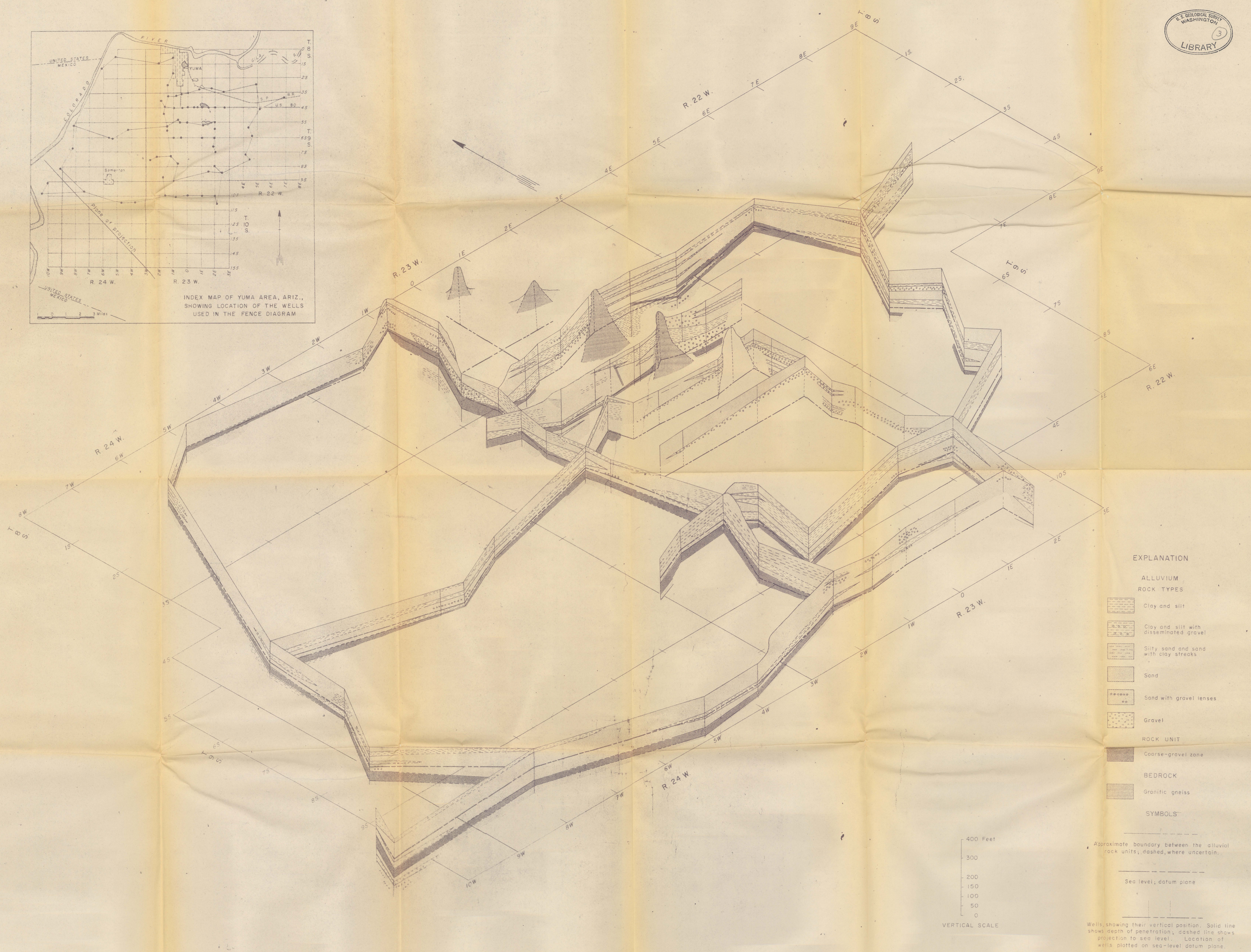
FENCE DIAGRAM OF THE SUBSURFACE ALLUVIAL ROCK UNITS IN THE YUMA AREA, ARIZONA
