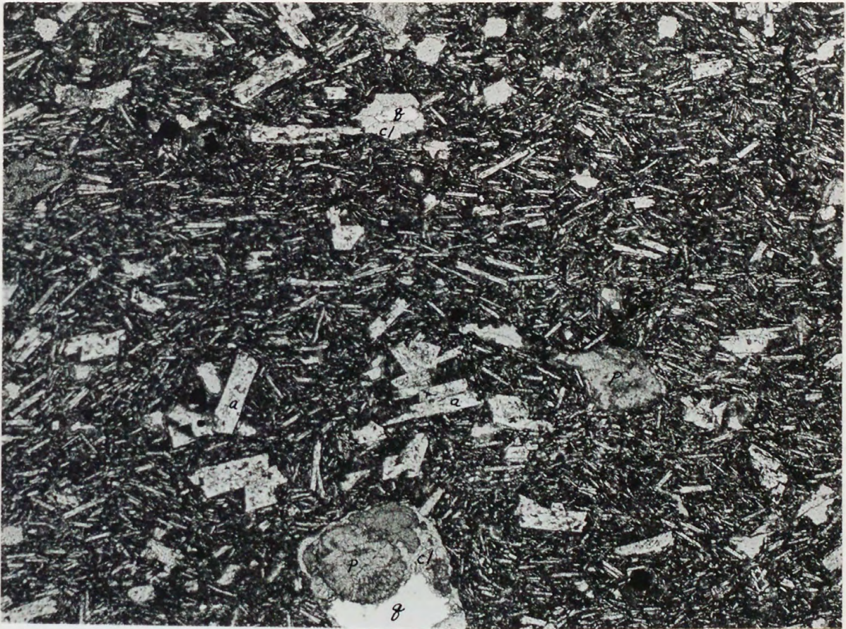
Figure 5--Photomicrograph of porphyritic amygdaloidal spilite with pilotaxitic groundmass. Principal minerals are albite (a) as microphenocrysts and groundmass lathes, chlorite (cl) as amygdule fillings and interstitial to albite in groundmass, pumpellyite (p) as amygdule fillings and interstitial to albite lathes, and quartz (q) which fills centers of some amygdules. Black grains are magnetite, which is disseminated throughout the rock. Some calcite is present (X 25).
