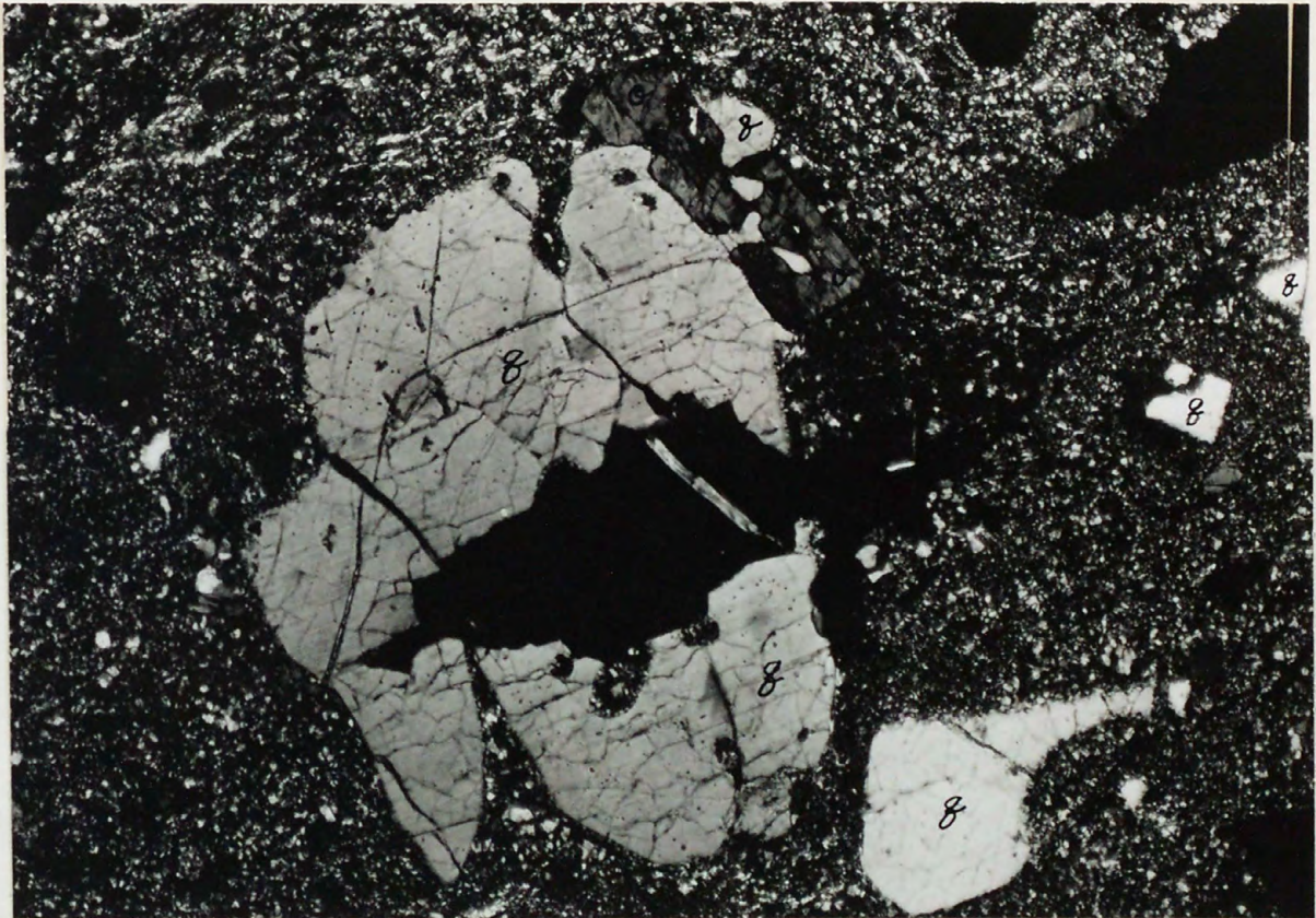
Figure 7--Photomicrograph of metadacite pyroclastic rock from southeast flank of Bully Hill. The phenocrysts are quartz (q), calcic oligoclase (O), and vermicular intergrowths of the two minerals. The vermicular quartz is interpreted as a replacement of plagioclase and is probably of late magmatic origin. The groundmass is chiefly xenomorphic microcrystalline quartz of hydrothermal origin; it locally replaces the plagioclase component of vermicular intergrowths, leaving vermiform quartz grains embedded in a groundmass of microcrystalline quartz that forms overgrowths on the vermiform quartz (X 50).
