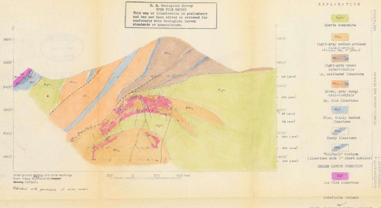
Plate 6:-Geologic section of the Independence mine showing stope outlines
