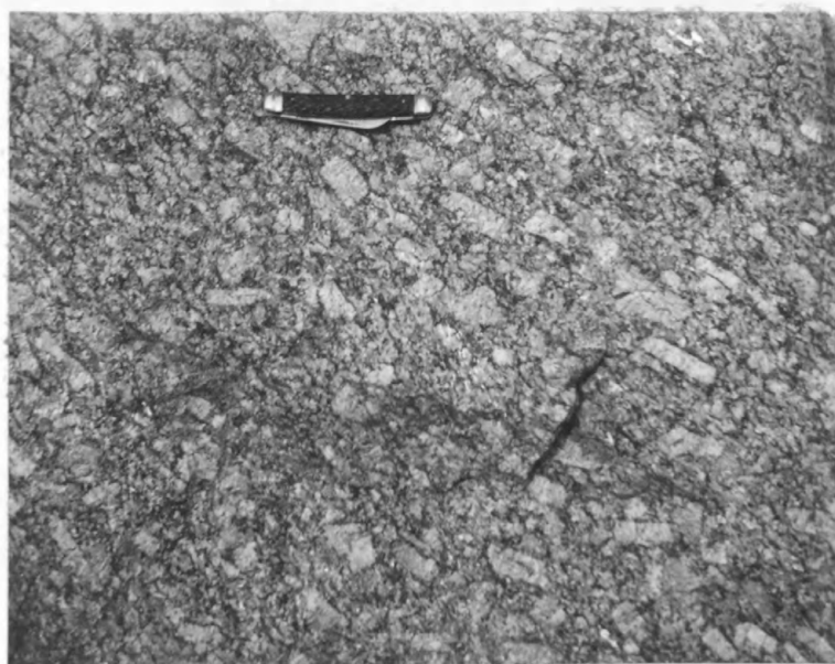
Plate 11. Photograph of typical Hoskin Lake porphyritic granite. Note the large, euhedral feldspar phenocrysts (light gray).
