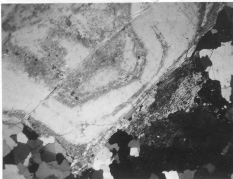
Plate 12. Photomicrographs of oligoclase phenocryst in Hoskin Lake granite. A. Note zonal arrangement of fine-grained sericite (gray) in sub-hedral oligoclase phenocryst (white). Quartz (white) and biotite (dark gray) are also present. Plane polarized light. x23. B. Same as A. Crossed nicols.
