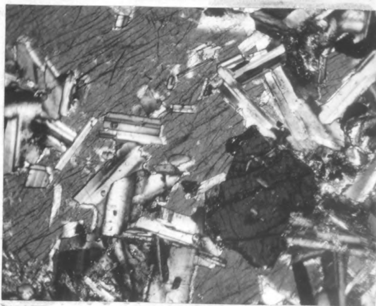
Plate 26. Photomicrographs of diabase. A. Plagioclase (light gray), pyroxene (medium gray, moderate relief), olivine (medium gray, high relief), and magnetite (black). Plane polarized light. x40. B. Same as A. Crossed nicols. x40.
