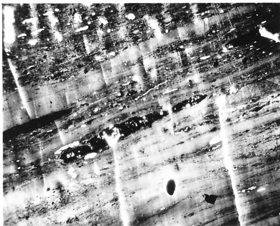
Figure 15. Photomicrograph of Sunnyside coal. Transparent clear bands are anthraxylon. Macerated bands are attritus. White spots are resin. This is bright coal or clarain.
