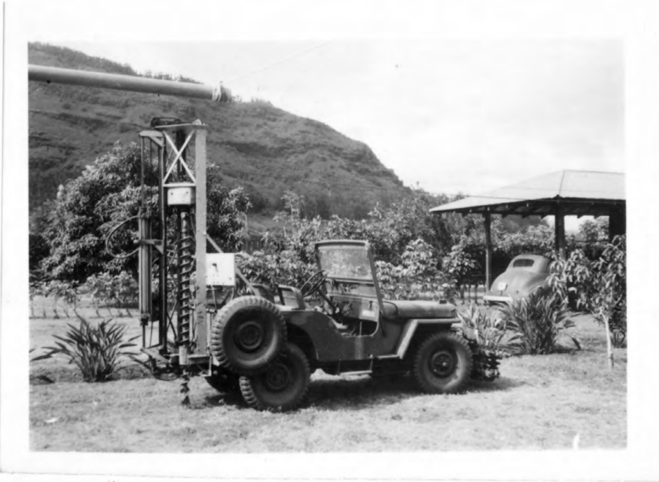
Figure 2. Jeep mounted mobile auger used in drilling for bauxite.
