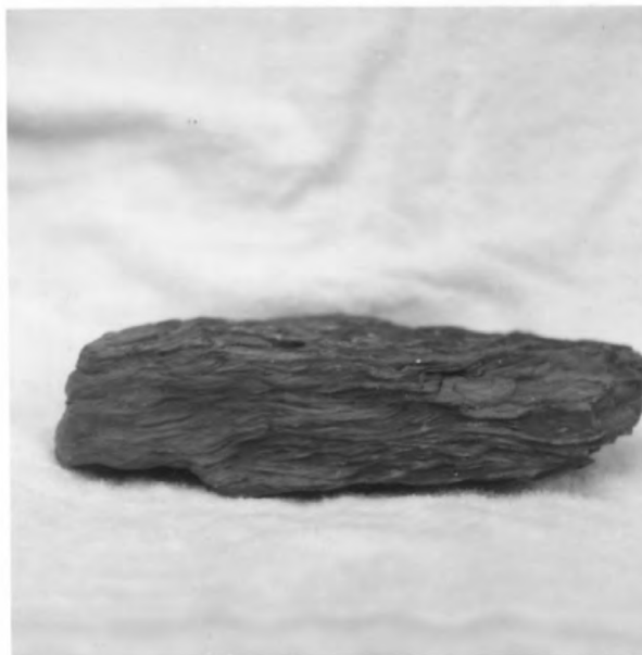
Figure 11.--Side view of rib-and-furrow structure from lower red member of Chinle formation in east-central Arizona (rock about 8 inches across)
