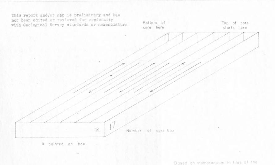
Figure I. Diagram showing arrangement of core in boxes,
